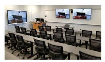
One side of the room is equipped with a SimplTrack camera to track the presenter. The other side has a 12X-SDI PTZOptics camera which connects to the Inogenie Share 2. This setup allows the professor and the audience to be captured for the video conference.
