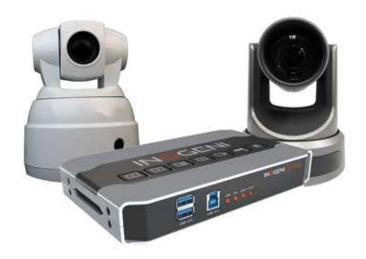
The Inogenie Share 2 is used to quickly switch between multiple cameras with the press of button. The Share 2 can bring together two camera sources in a variety of outputs and connect to Zoom Video Conferencing with a single USB 3.0 cable.
